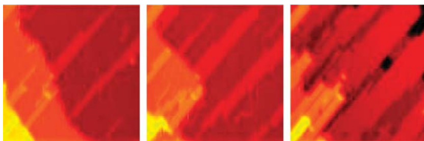
Fig. 3 Snapshots from an STM movie showing a Cu(110) surface during exposure to \sim 10^{-8} Torr O_2 at room temperature. The removal of Cu atoms from step edges is accompanied by the nucleation of added rows in the [001] direction.
